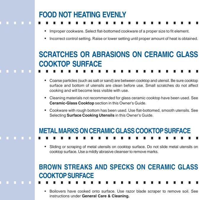
• Cleaning materials not recommended for ceramic-glass cooktop have been used. Use recommended cleaners and cleaning method. See **Ceramic-Glass Cooktop** section in this Owner's Guide.
